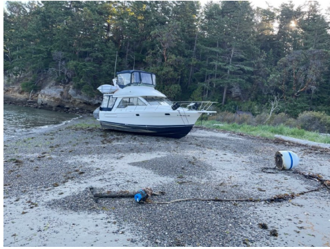
Anchor failure resulting in moored boat washing ashore at Sucia Island.
