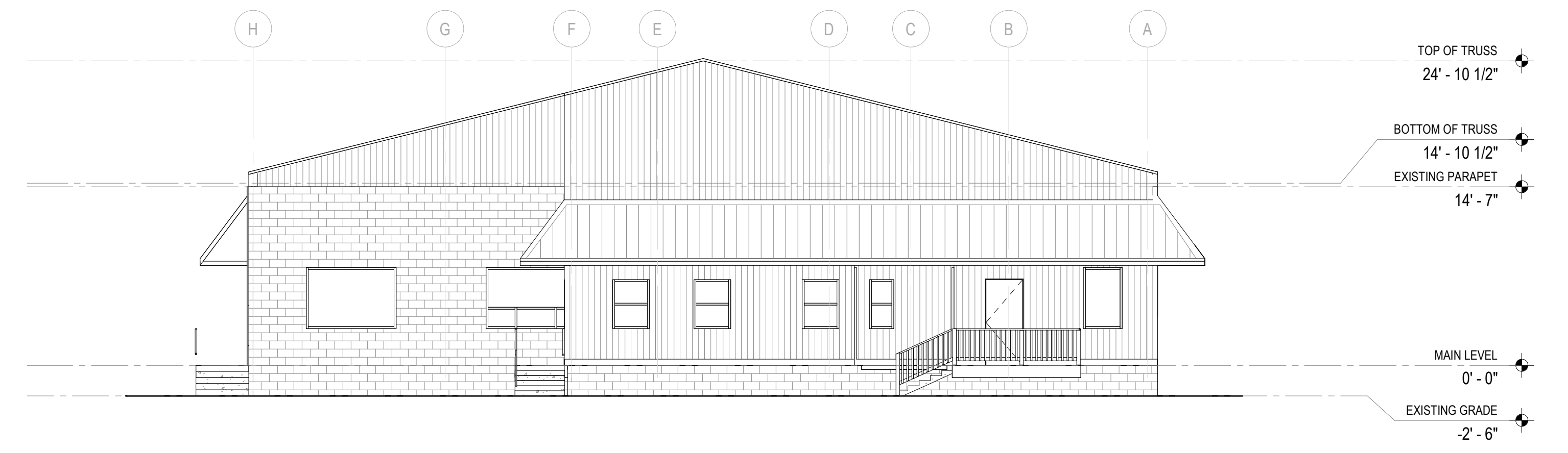
2 NORTH ELEVATION - DEMO/ NEW SCALE: 1/8" = 1'-0" NOTE: FOR REFERENCE ONLY, NO WORK ON NORTH FACADE
